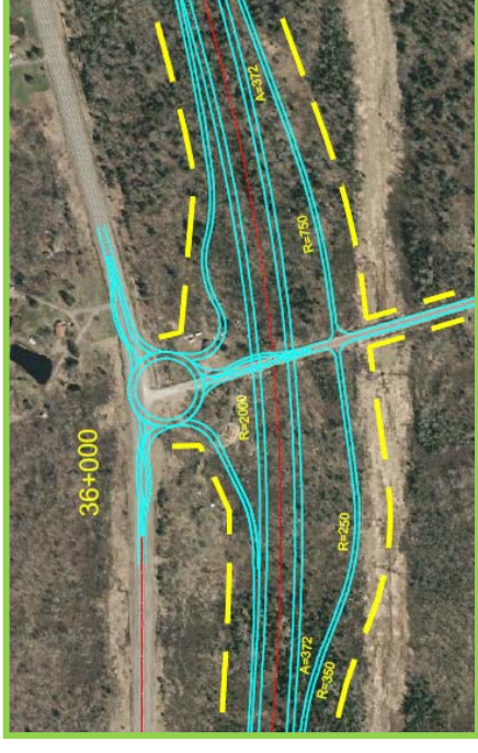
Boundary Road Interchange Diamond - Roundabout Configuration
